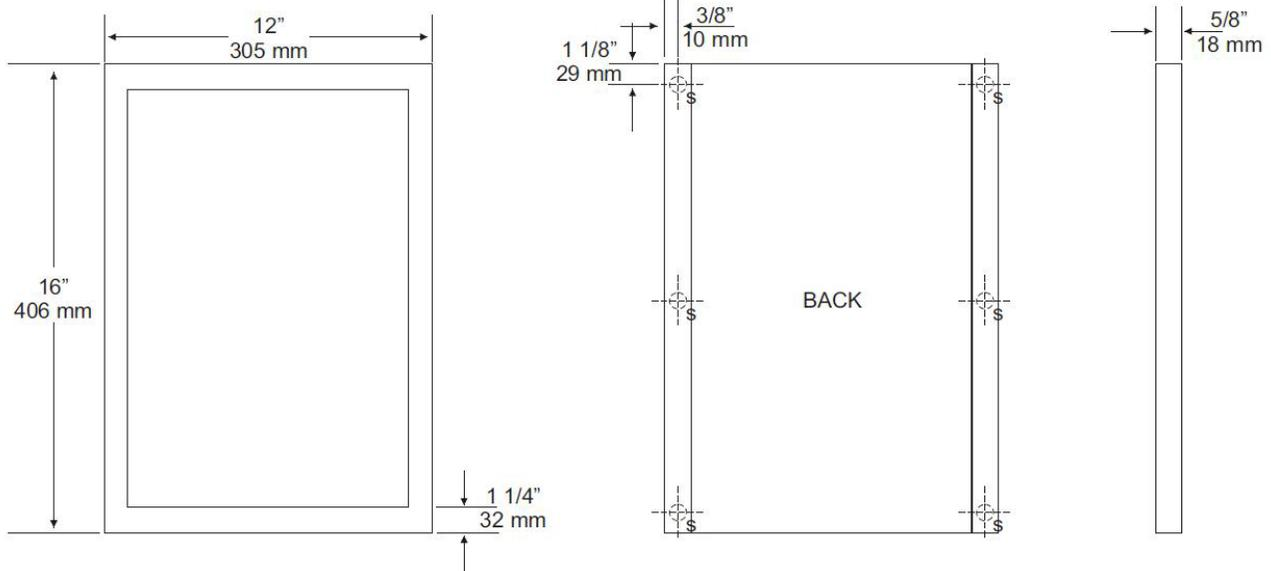
**Frame:** Fabricated of type 304 #14 gauge stainless steel with a #4 satin finish. (1 1/4" x 5/8") Welded construction with polished edges without miters.
